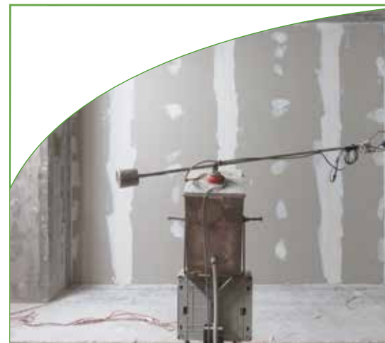
Airborne sound laboratory test Trocellen false wall
